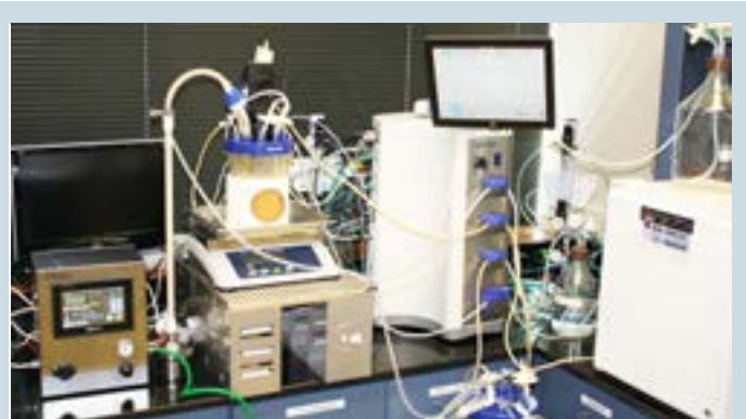
Fig. 8: Connection of the BioFlo 320 bioreactor control station with ATF cell retention device
