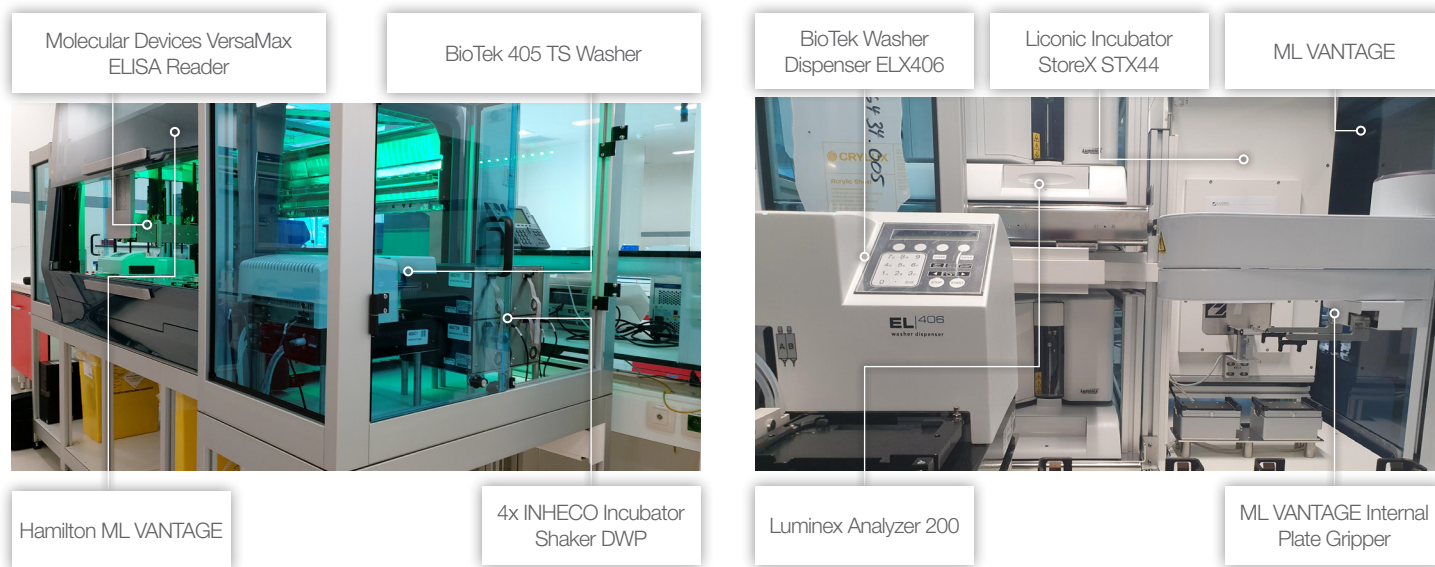
Figure 6: Two Examples of the Integration of Hamilton platforms with Third-Party Instruments for LBAs. Photos were taken by Hamilton Application Specialists during system installations.
