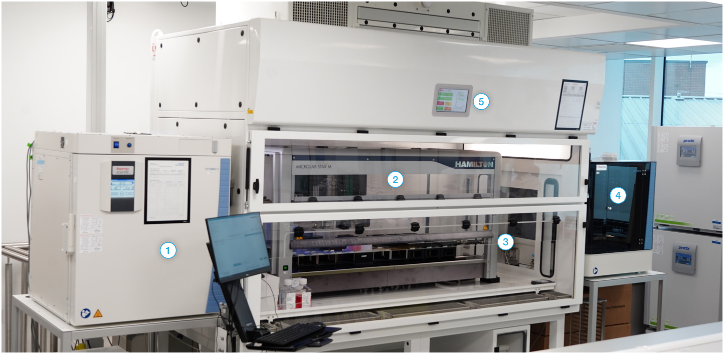
Figure 1. System Overview. (1) Cytomat™ 5 C Automated Incubator, (2) Hamilton Microlab® STAR™, (3) Linear Track, (4) Cytomat™ 10 Hotel, (5) Contained Air Solutions Class II Cabinet.
