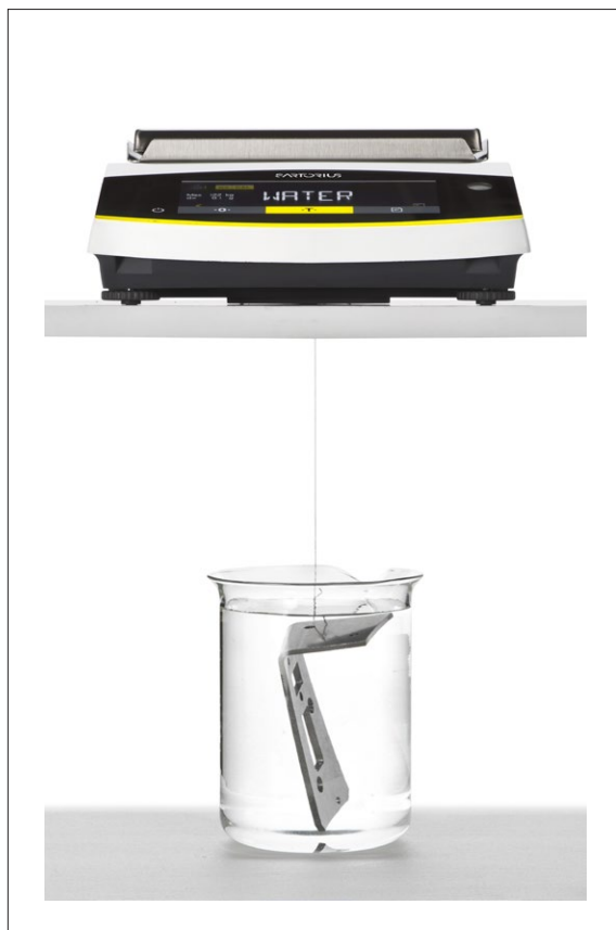
Figure 2: Below-balance weighing for magnetic samples with an Entris II precision balance
