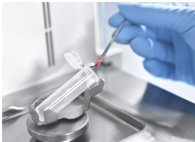
Figure 4: Titanium vial holder for a Cubis® II semi-micro balance reduces magnetic influences
