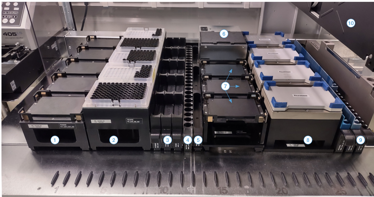
Figure 3. Deck Layout of the Customized Microlab® STARlet used for the Purity Tests. (1) Carrier for Deep-Well Plates used as lid parking position, (2) Tip Carrier, (3) 60 ml Trough Carrier, (4) 15 ml Tube Carrier, (5) 120 ml Trough Carrier, (6) Cooling Module, (7) 3X Deep-Well Plate positions, (8) Carrier with 4X Plate Shakers (Variomag), (9) Carrier with adaptors for 1.5 ml tubes, (10) 8X 1000 µl Pipetting Channels.
