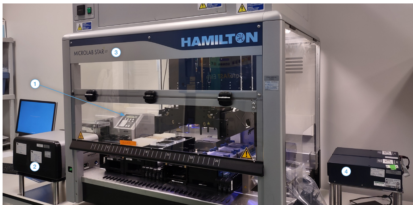
Figure 2. System Overview. (1) Biotek ELx405™ Select Deep Well Washer, (2) Biotek Epoch2® Microplate Spectrophotometer, (3) Hamilton Microlab® STARlet, (4) Inheco Single Plate Incubator Shakers
